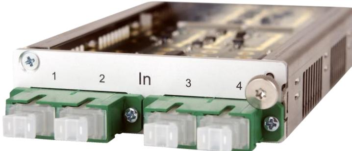
The Alpha Optical Receiver provides 4 optical input channels.
