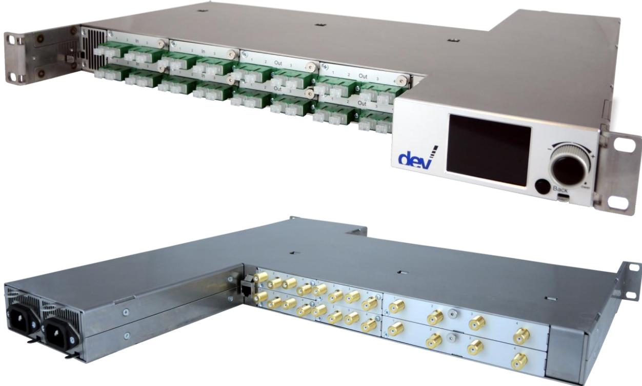
The 1 RU chassis can be equipped at the front side with up to eight optical modules, i.e. up to 32 optical channels. The RF ports (with and without redundancy functionality) installed at the rear side are assigned to the opposite optical module at the front side. In addition, the chassis is equipped with a redundant power supply, provides a local user interface, the DEV Web Interface, and SNMP support.
